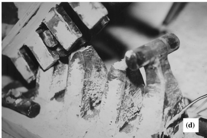
FIG. 2. Ductile End-Diaphragm Specimen Having TADAS: (a) Elevation; (b) Hysteretic Curves; (c) Plates under Considerable Flexure at 2% Drift; (d) Close-Up of Device after Experiment
