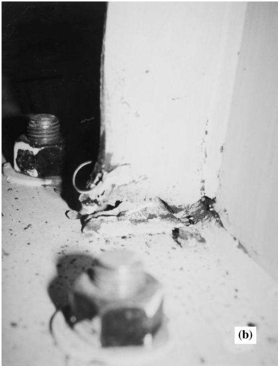
FIG. 3. First Specimen without Diaphragm: (a) Hysteretic Curves; (b) Fracture of Full Penetration Welds at Bottom of Girder Bearing Stiffeners
