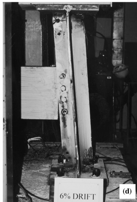
FIG. 8. Nonductile Nominal Diaphragm Specimen: (a) Photo Showing Deep Channel at Midheight between Stubgirders; (b) Hysteretic Curves; (c) Rupture of Top Bolt on West Side; (d) Subjected to Drift of 6% Also Showing Two Ruptures of Bolts
