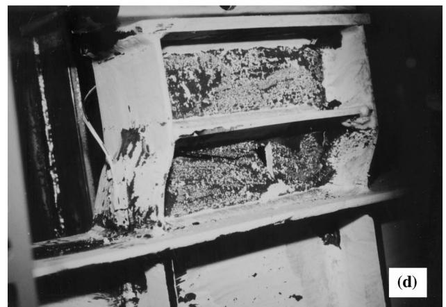
FIG. 6. Ductile End-Diaphragm Specimen Having SPS1: (a) Elevation; (b) Hysteretic Curves; (c) Link Visible Buckling in Flanges and Deformation as Parallelogram Bounded by End Plates and Flanges; (d) Fracture Propagation through Web of Link
